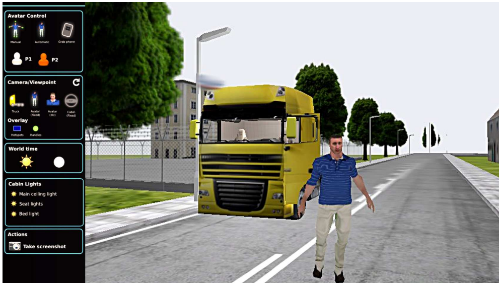
Figure 5.3 A screenshot of the application prototype. The avatar represents a persona and can be used to act out use scenarios in the virtual world. The on-screen user interface (on the left) was introduced after reviewing the first prototype, and provides access to common world settings, camera viewpoints and avatar actions.
